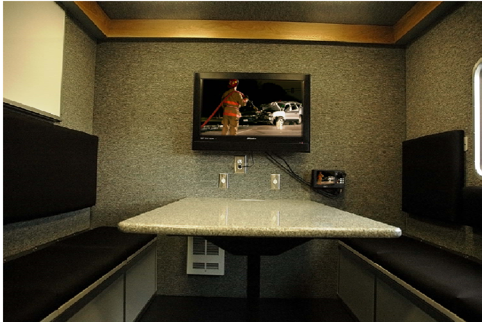
Private conference center with 36" wide solid-surface table. Four-man bench seats on each side wall with storage beneath. Ninth person can sit at head of table. 32" LCD monitor on back wall with remote control for Nightvision camera. Note wiring access around ceiling perimeter for ease of subsequent integration.
