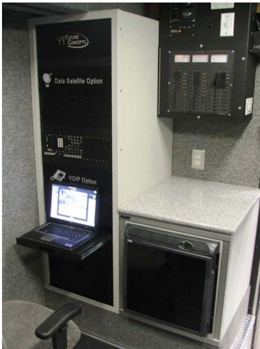
37RU Electronics rack ready for installation of communications equipment. Refrigerator with solid-surface work counter next to side entrance door.
