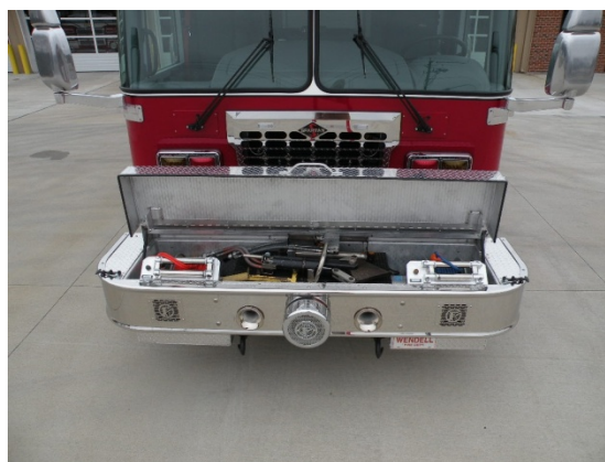
A hydraulic hose reel and utility air hose reel are mounted in the front bumper. A Hurst Combi-Tool is pre-connected to the hydraulic reel.
