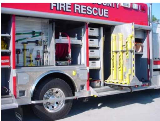
Air shores are mounted on a slide-out rack that extends fully out of the 40" deep compartment. Note tool board in front of water tank.
