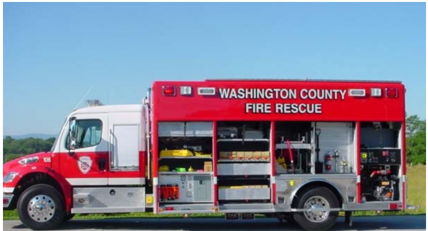
Shown with 25kw PTO generator in left front and 300-gpm Darley pump in left rear compartment. Note booster reel forward of 250 gallon water and foam tank with tool board on face of tank. The two 10" high slide-out trays in the second compartment are 38" deep and hold all cribbing for fast deployment. The upper left front compartment features a tunnel for four long backboards.
