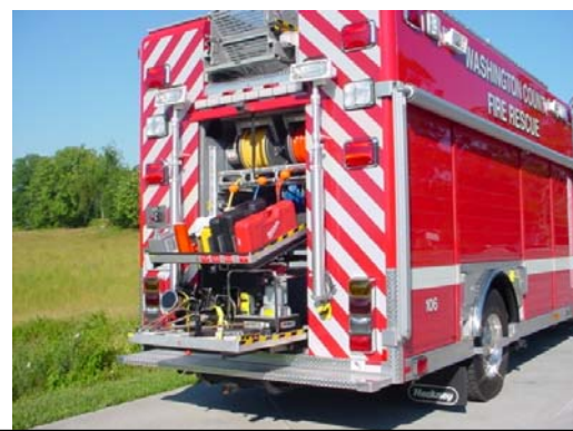
The rear extrication tool compartment carrying all hydraulic tools, electric saws and air chisels. Note the hydraulic hose, utility air and electric cord reel in the top of the compartment. A slide-out captive roller assembly permits deployment down either side of the apparatus. The electric awning deploys rapidly for use as a rehab station and during incimate weather.
