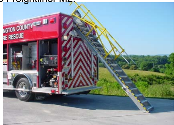
The Auto Deploy Staircase (ADS) provides safe access to and from the roof storage compartments.
