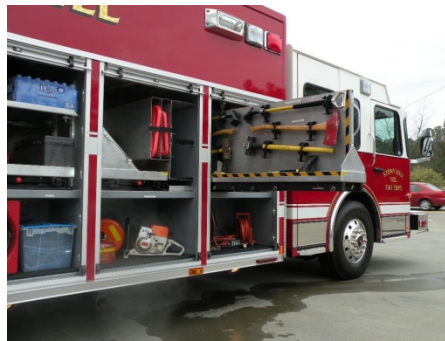
Slide-out tool board and other slide-out rack/trays facilitate access to equipment.
