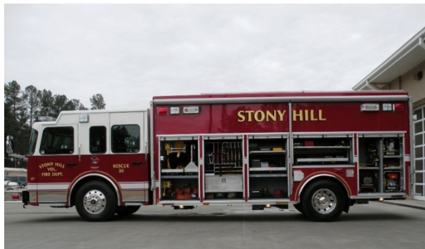
SCBA's can be refilled off the on-board cascade system. The four DOT storage cylinders are mounted against the back wall behind the fill enclosure. Three 36" deep full height tool boards, slotted air bag storage and eight spare SCBA bottle storage tubes compliment the curb side of the body.
