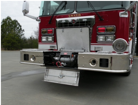
9000# portable winch stores in the front bumper ready for use in a 10,000# receiver. It can be relocated to either side or rear of the body.
