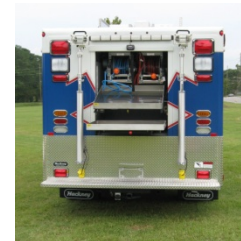
Rear extrication tool compartment with two hydraulic reels.
