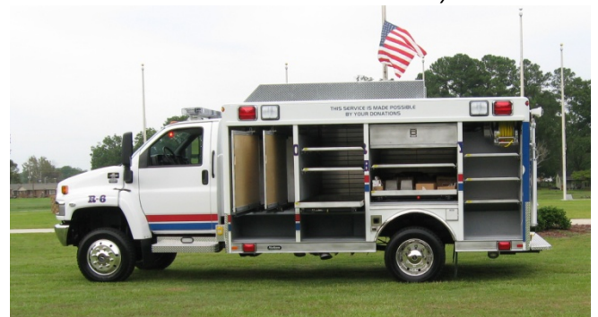
Two 65" deep slide-out tool boards in the front and transverse tunnel compartments for stokes basket and two long back boards enhance storage convenience.
