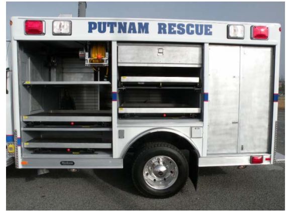
STREETSIDE: Transverse tunnels in the upper wheelhouse house a stokes basket and two long back boards. Cribbing is stored behind hinged doors in the left rear.
