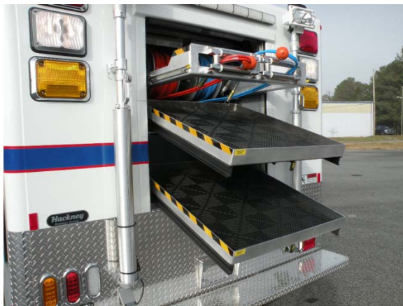
REAR: Slide-tilt trays provide storage for extrication tools. Note the slide-out hydraulic hose roller guides facilitating deployment of hoses out either side of the body.
