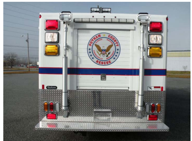
Because of foggy conditions along I-40, extra LED warning lights were added to the rear; traffic director light bar; four upper warning lights and two lower warning lights, all LED. The removable tripod flood lights can be used while on the vehicle or remotely when connected to the cord reel.
