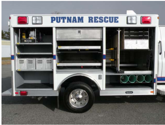
CURBSIDE: Note special storage slots for air bags and controls in upper front compartment. A 64" deep slide-out tool board provides plenty of storage for SCBA and hand tools.
