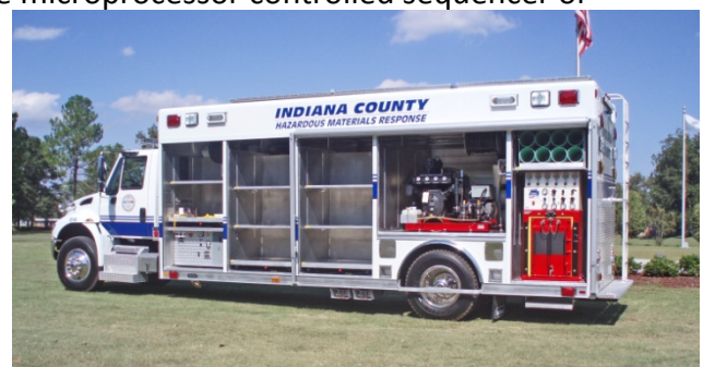
A 26.5 cfm breathing air compressor and RevolveAir fill station provides on-scene air support operations. Not cavernous storage compartments for hazmat equipment.
