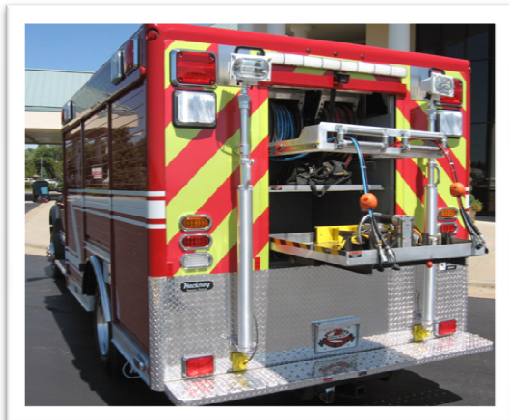
The rear compartment is dedicated to the hydraulic rescue tool compliment. Note the slide-out hose roller guide for the two hydraulic hose reels.
