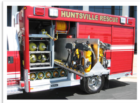
Plenty of breathing air on-board with a two-bottle fill station on the curb side, six complete SCBA's on a slide-out rack with "back-up and go" donning and spare SCBA bottle tubes on the lower floor.
