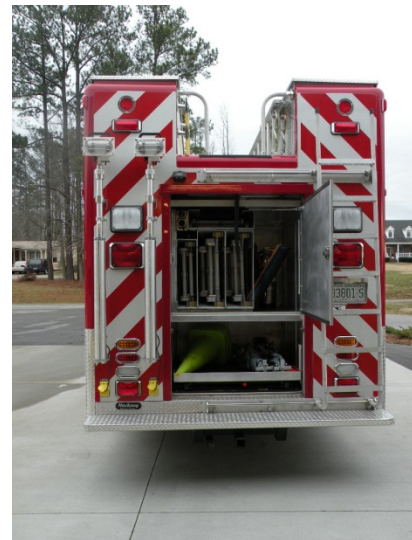
Rear compartment accommodate a full ladder compliment and pike poles. Roof access ladder slides to the center position
