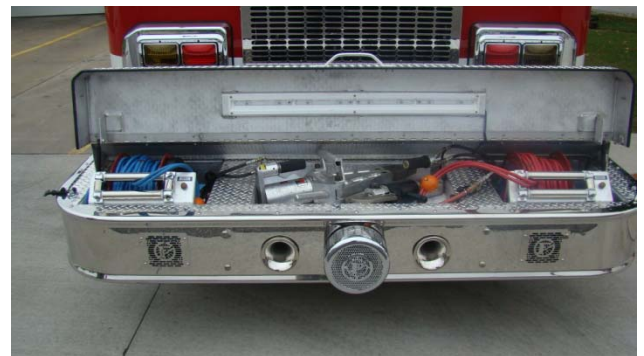
Two pre-connected hydraulic rescue tools are stored in the front bumper.
