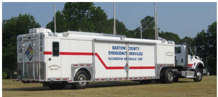
An observation platform is installed on the roof with rapid deployment design. Rear science lab and command center is access through the side entrance door.
