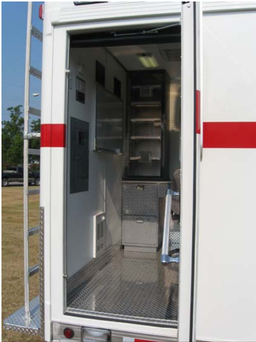
The Science and Command Compartment features "L" shaped cabinets and desk to maximize utilization of space. Two-drawer filing cabinet and testing equipment storage cabinets are in the rear corner.
