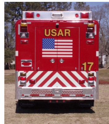
The rear tunnels store 12-ft timbers and shoring panels. Note the drop-down bumper step platform.
