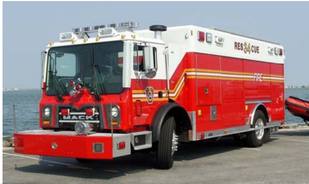
The severe-duty front bumper includes a drop down door that accesses a portable winch that is stored and also used from this location.
