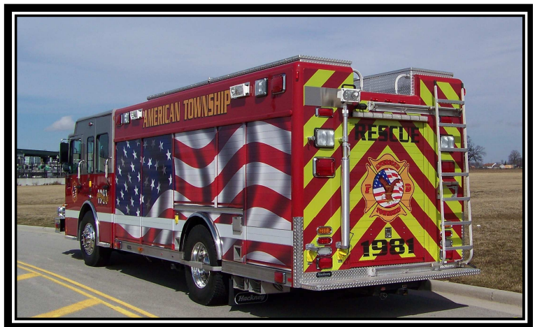
A sliding "Library" ladder parks out of the way of the rear extrication compartment when not in use. The extrication tool compartment is a full 64" high x 40" deep.
