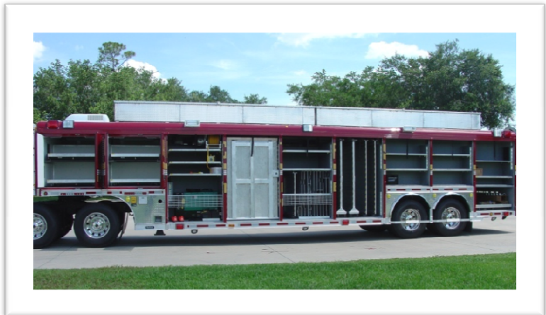
Drop-down ramp in #4 compartment allows the Stanley tool to be rolled directly into and out of the compartment. Vertical slide-out boards in #6 are dedicated to airshores.
